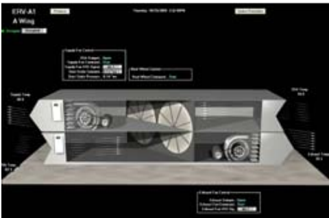
An energy recovery ventilator (ERV) unit is installed in each wing of the school to increase indoor air quality and reduce energy costs.
