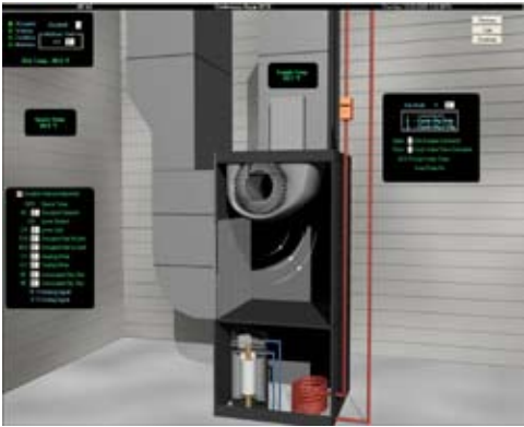
Customizable BACtalk displays show comprehensive, real-time data; in this example, a heat exchanger visual shows temperatures for outside air and supply air.
